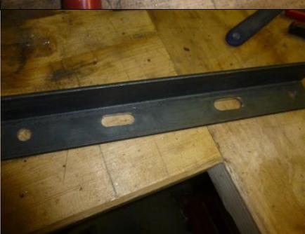
A photograph showing a metal plate being cut with a hand saw. The plate is resting on a wooden workbench and has several holes already drilled into it. A hand saw is being used to cut along the length of the plate. | <p>Mit der Sticksäge werden die Löcher der Motorenhalterung verbunden; damit man später den Motor auch an die richtige Stelle schieben kann.</p> |
