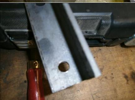
A photograph showing a metal plate being drilled. A red-handled drill is being used to drill a hole into the plate. The plate is resting on a wooden workbench.                                                        | <p>In die Eisen der Motorenhalterung musste ich je 6 Löcher bohren.</p>                                                                          |
